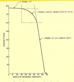
Fig. 1. Transmittance of window glass.
